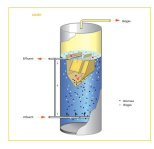
The technology applied in the UASB + reactor is a method of anaerobic digestion of the organic load of wastewater, resulting in biogas and granular sludge (granules) production. The reactor is named after the upward flow of the raw wastewater, through an anaerobic sludge layer, in which anaerobic microorganisms are grown, that break down the waste. This layer of sludge that tends to settle, in conjunction with the upward flow of wastewater, creates the conditions for
