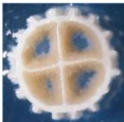
Detailed view of the carrier with the biomass developed in its protected surface
